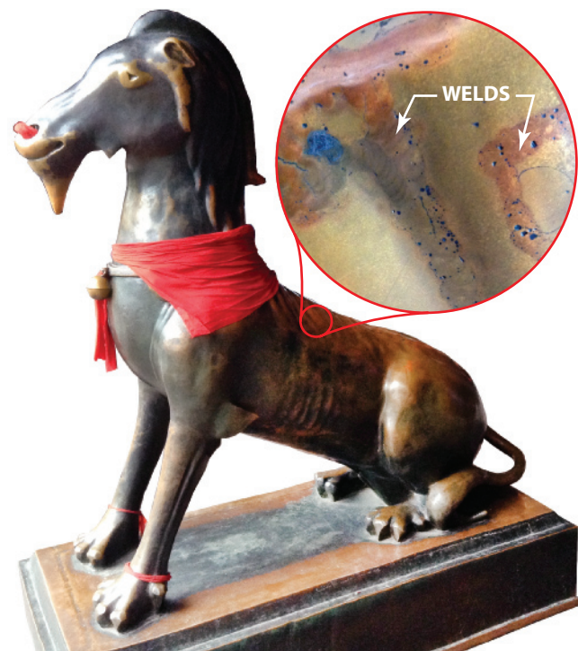
FIGURE 1-3 Bronze goat statue in Chengdu, China cast more than 1,500 years ago and repaired with braze welding about 1,000 years ago.
